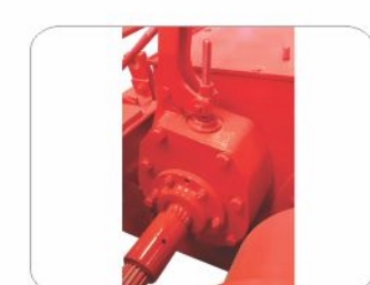
Oil-immersed brake designed for use on a drive heavy machines
